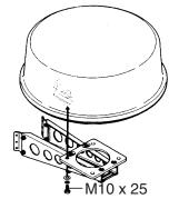
(B) Fastening antenna to mounting bracket
