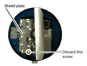
Antenna unit, cover removed, top view
