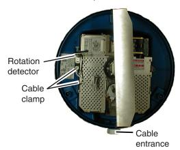
Antenna unit, cover removed, top view
