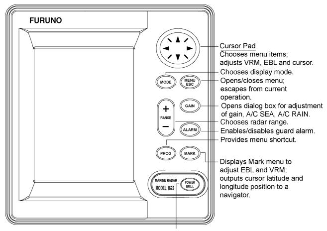
**Short press:** Turns power on. **Long press:** Turns power off.
