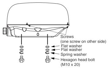
Antenna unit, showing location of mounting hardware
