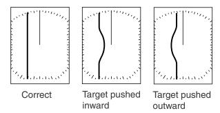
Improper and correct sweep timing
